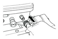
3 Install a lock in the stop switch.
