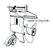
3 Install the upper oil plug, and then remove oil tube nozzle and install the lower oil plug.
