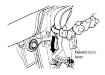
2 Return to normal running position: Put the reverse lock lever in the tilt down position, slightly lift up the outboard motor, and then put it down.
