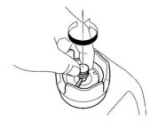
**2** Connect the fuel connector to the engine.
