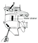
2 Insert the oil tube nozzle into the lower oil plug hole, and fill with gear oil by squeezing the oil tube until oil flows out of the upper plug hole.
